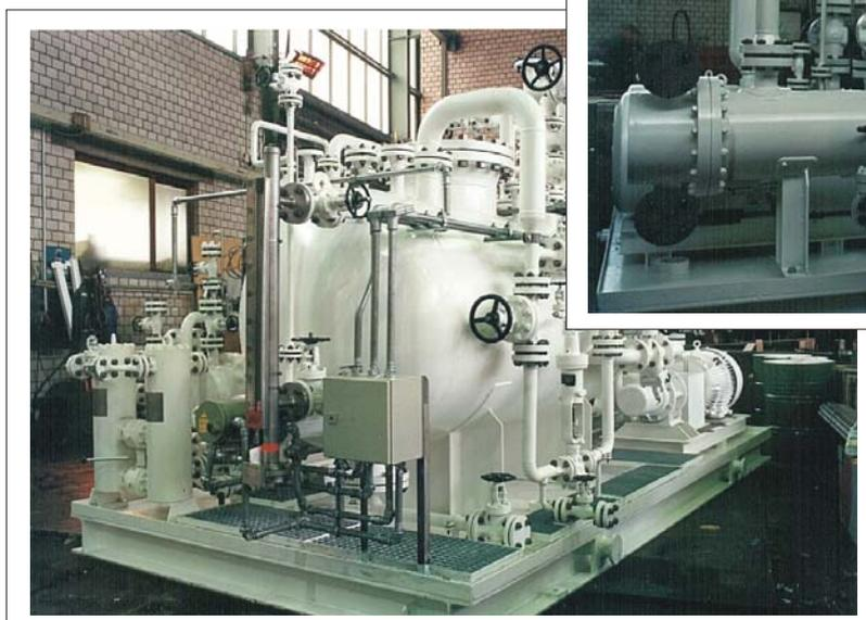
The seal oil system as the complementary part for the process pump shows the vessel shaped reservoir indicating a higher operating pressure than the lube oil system.
