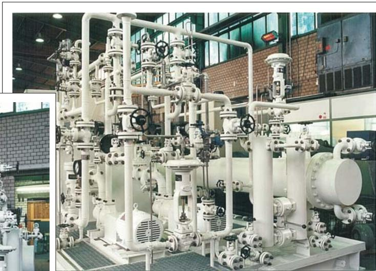
The pictures show a lube oil system on a separate console for a process pump for a major global chemical company. Installations in Argentina, the United States and the Netherlands are successfully operating. Further projects all around the world are planned. **OELTECHNIK** assures that all international and national code regulations are followed.
