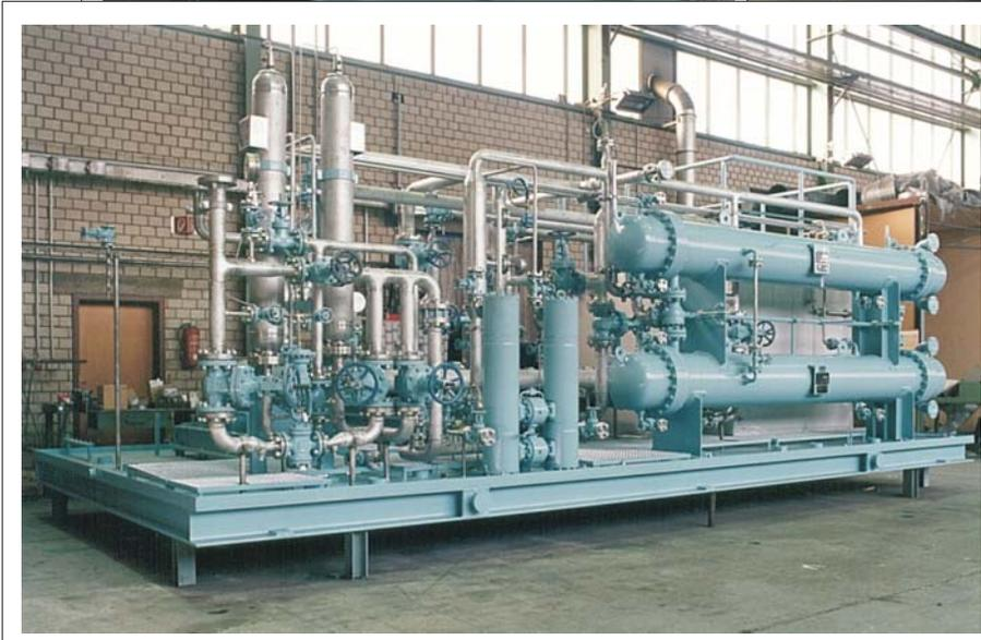
**OELTECHNIK** designs and fabricates oil systems according to customer`s specification. The combined lube and control oil unit for a centrifugal compressor shows a special anchoring system under the base plate for installation in seismic zones. The rigid base plate shows lifting lugs to ease handling of the console.
