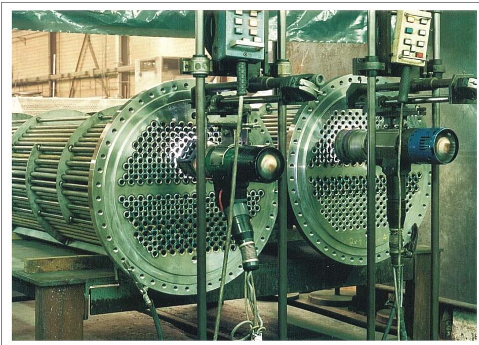
**OELTECHNIK**'s full automatic orbital welding equipment welds tube to tube sheet joints to a highest degree of perfection. All welding parameters entered by the certified welder based on the WPS (Welding Procedure Schedule) are stored on micro chip. Therefore a high level of welding quality is assured for every single tube joint on the tube bundle. For multiple weld layers each pass is checked for cracks and crevices by a Liquid Penetration Test (LPT).
