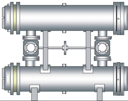
For oil systems with high availability requirements, **OELTECHNIK** offers the twin cooler assembly including continuous-flow transfer valves. Each oil cooler is designed to handle 100% oil flow. The flow can be switched from one cooler to the other with the help of two transfer valves connected to shell side oil in- and outlet. Tube side fouling on the oil cooler which is not in operation can be removed without causing any downtime of the system.
