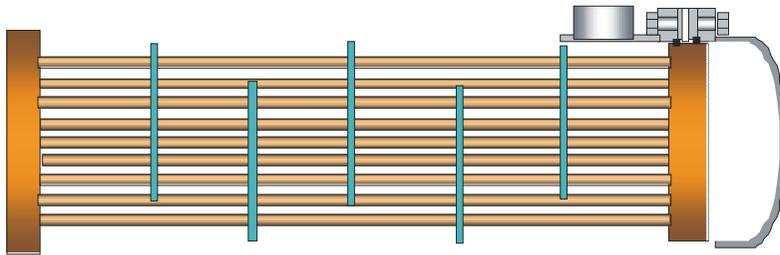
**OELTECHNIK's** TEMA Type **BET** is only used for even pass numbers on the tube side. In- and outlet connections of tube side are therefore on one side. The integral bonnet has to be removed in order to have access to the tubes on the floating end of the bundle.
