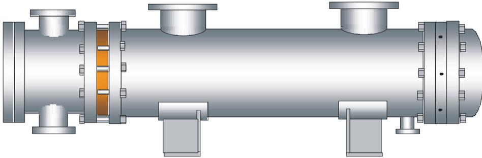
The baffles lead the shell side fluid across the tube bundle. Baffle spacing and percentage cut are selected in the rating process to allow for optimum flow conditions during operation. Heat transfer aspects and vibration prevention aspects are considered to find the optimum solution.
