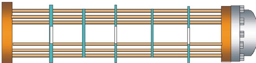
**OELTECHNIK**'s TEMA Type **BEW** is mostly used for gas through the tubes and water on the shell side. The flow arrangement is counter-flow, cold water cools colder gas, warmed up water cools incoming hot gas. The tube and shell side are one pass, respectively. The bonnet can be designed as shown with axial connections or radial connections.
