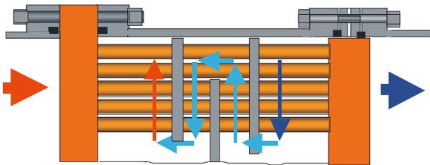
The stationary tube sheet is clamped between shell flange and water bonnet. The floating tube sheet slides in the external seal formed by shell flange and rear bonnet. Regular segmental baffles guide shell side fluid through the shell.
