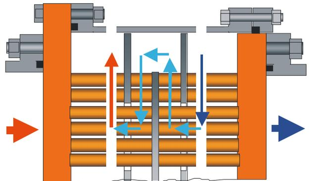
The tube to tube sheet connection is a critical joint which is exposed to both shell side and tube side fluid. It has to be tight against leakage and as a pressure bearing part it has to be resistant to stress and forces. Tube and tube sheet can be of different material or the same kind. The type of joint design which is the most efficient is a function of material combination, design pressure, design temperatures, and tightness requirement.
