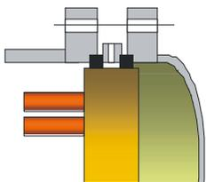
The TEMA type **AEW** seals floating tube sheets externally with two rubber packings. The support disc shows leak detection lines to immediately indicate dysfunctional seals prior to leakage to the other fluid system. The TEMA type **AES** (figure on the right) seals the tube side against shell side with a floating head held by a backing ring.
